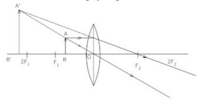
3. A convex lens forms a real and inverted image of a needle at distance of 50 cm. from it. Where is the needle placed in front of the convex lens if the image is equal to the size of objects? Also, find the power of lens.
