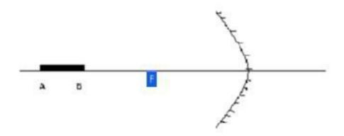
21. A rod of length 10 cm lies along the principal axis of a concave mirror of 10 cm in such a way that the end closer to the pole is 20 cm away from it. Find the length of image?
